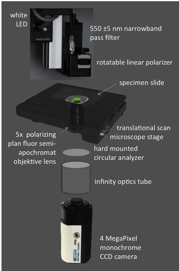
Fig. 3 – Hardware setup of the polarization microscope.
