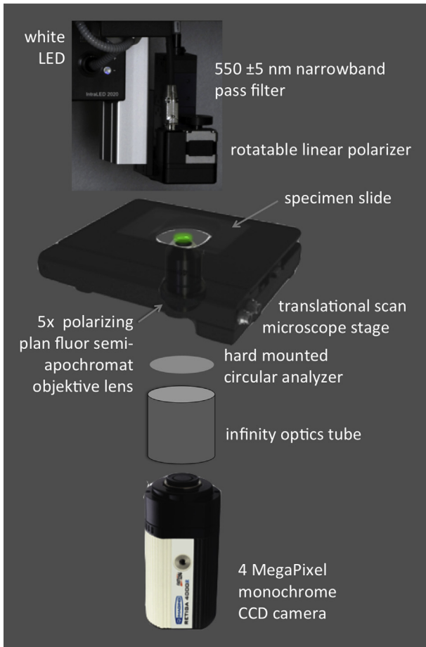
Fig. 3 – Hardware setup of the polarization microscope.
