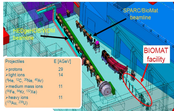
Figure 18: Layout of the future BIOMAT cave that will be used at FAIR for the biomedical applications within the APPA experiment. The vault includes the beamline for plasma physics and the SPARC experiment. Maximum energies of the beam that will be transported in BIOMAT are indicated in the insert.
