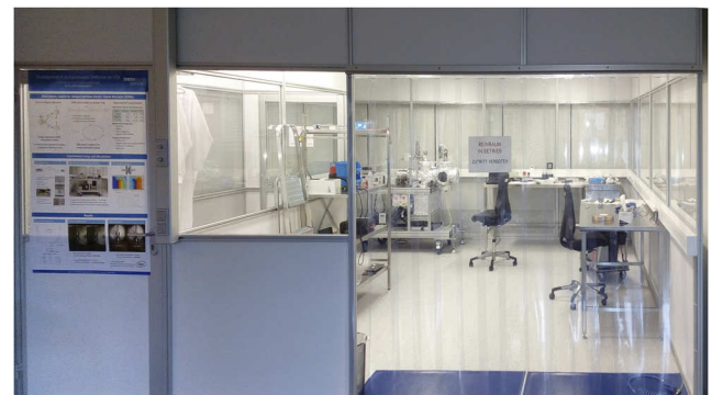
FIG. 3. Class ISO7 21 clean room at RWTH Aachen University, housing the experimental setup for electrostatic tests.
