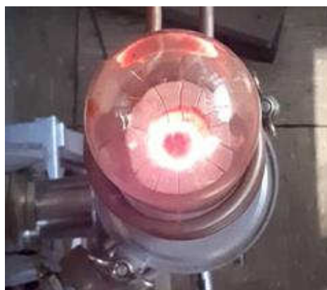
Figure 5.1: Photo of a crucible at the beginning of the melting process.
