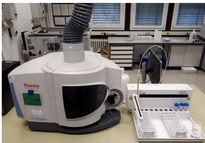
Figure 5.2: Photo of the used instrumentation for chemical analysis (iCAP 7600 ICP-OES).
