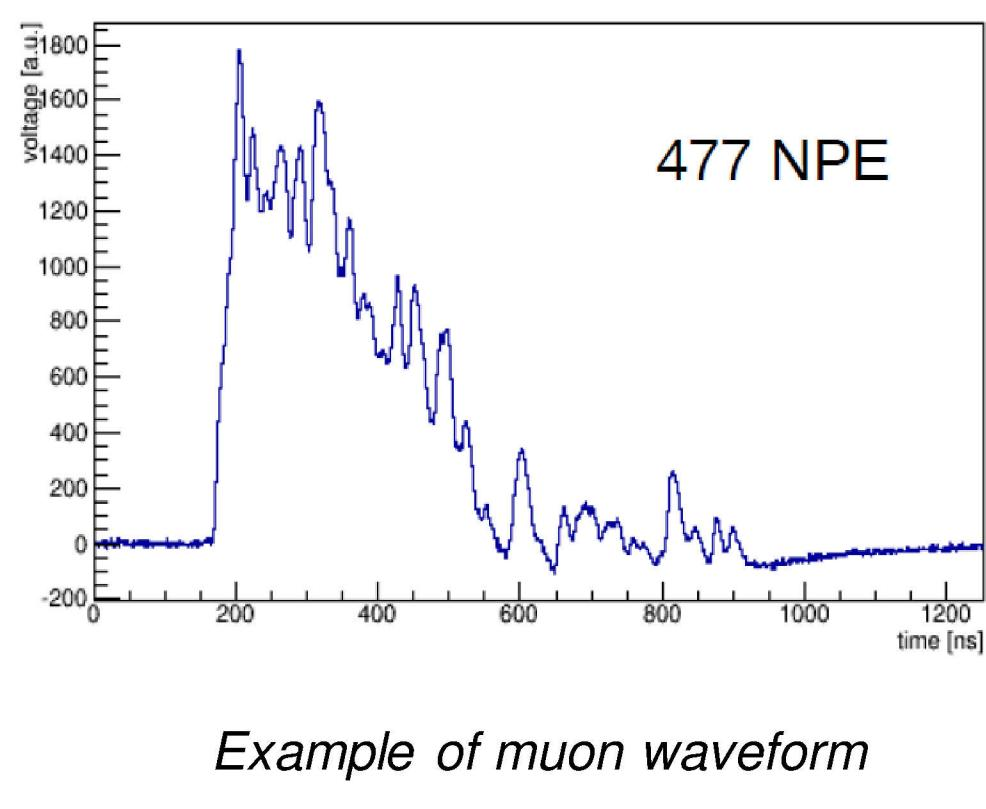
Example of muon waveform
