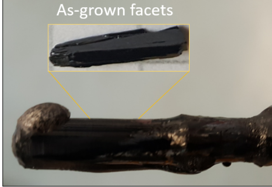
Figure 2: Crystal boule grown in gas flow of \text{CO}_2/\text{CO} = 33 and (001) facets
