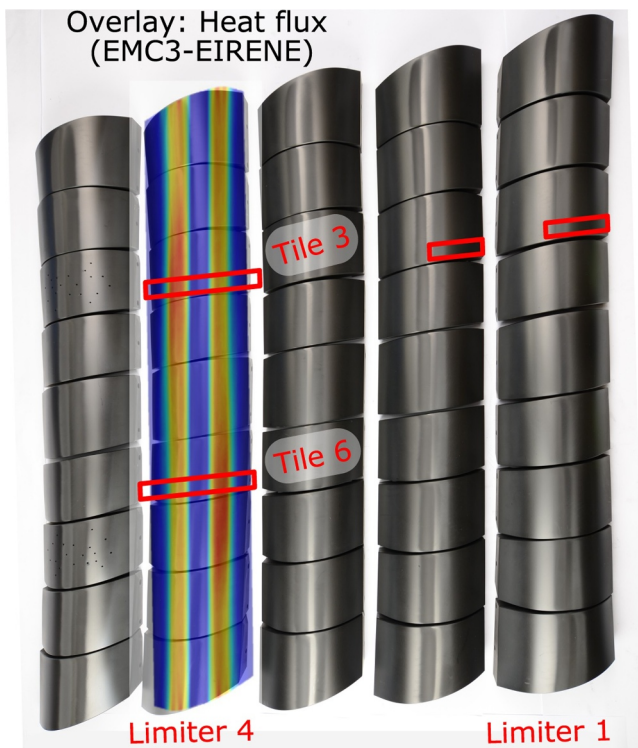
Fig. 1. Photo of limiter modules 5 to 1 (left to right), each containing nine tiles. Analyzed tiles are marked in red. On limiter 4 a simulation of the heat flux (EMC3-EIRENE code [13]) owing to electron and ion impact is overlayed. (For interpretation of the references to colour in this figure legend, the reader is referred to the web version of this article.)
