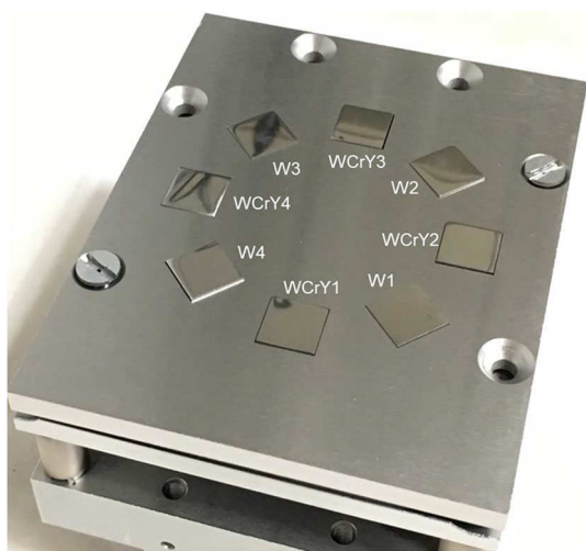
Fig. 2 Target holder with radially placed WCrY and W samples for exposure in PSI-2
