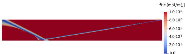
Fig. 6. TC1: ^4\text{He} concentration at steady state. Maximum computed ^4\text{He} concentration is 1.2 \cdot 10^{-2} \text{ mol/m}^3_w .
