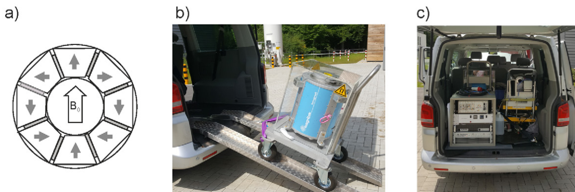
Fig. 1. The transportable Magritek magnetic resonance imaging (MRI) tomograph built of permanent magnets: (a) schematic drawing of one ring-shaped Halbach array with main building block magnets and shim magnets (gray)—several of such rings are stacked to form the entire magnet; (b) the tomograph is mounted on a vibration-damped trolley; and (c) the instrumentation including magnet, spectrometer, chiller, and amplifiers can be transported easily in a small van.
