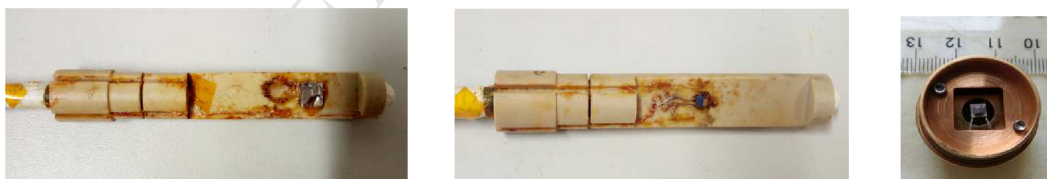
Figure 2: The holder for the direct measurements of the MCE with the samples mounted on it (left), the back side of the holder with the reference junction installed (middle) and the holder for the heat capacity measurements with the sample on it (right)
