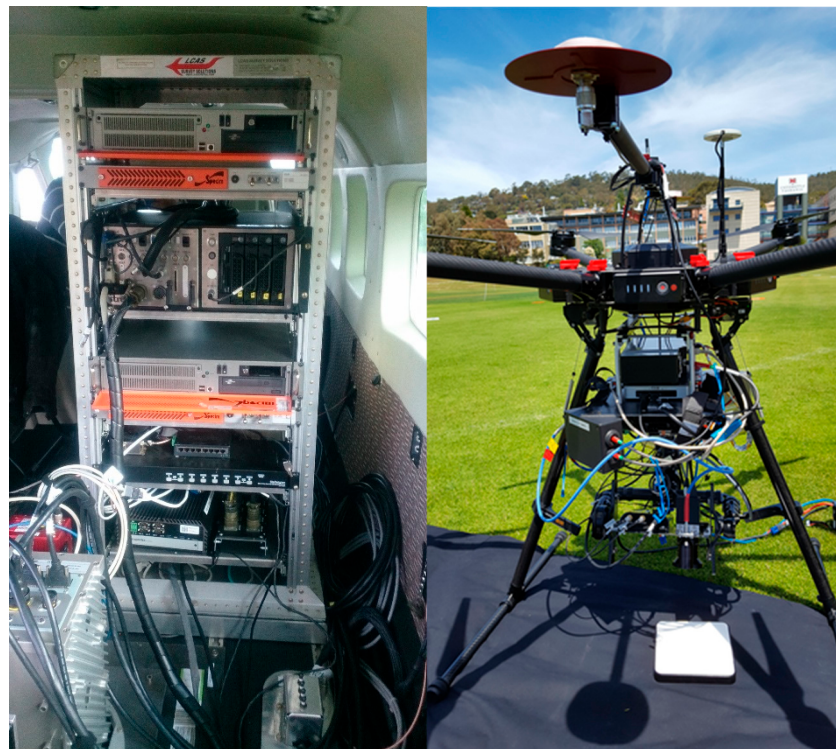
Figure 5. Two different F sensors installed on different platforms: HyPlant installed in an aircraft ( left ) and AirSIF system [95] with QE pro of the Terraluma group installed on a multirotor UAV ( right ).
