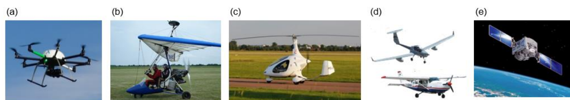
Figure 3. Different air- and spaceborne remote sensing platforms for assessing geodiversity and geotraits, (a) unmanned aerial vehicles (UAV, or drone), (b) microlight-gravity-controlled (c) gyrocopter-microlight helicopter, (d, top) Ecodemonia, (d, bottom) Cessna, (e) satellite.
