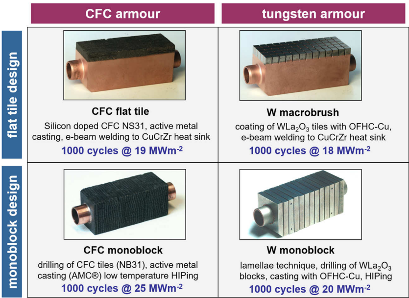
FIG. 8. Thermal fatigue experiments on CFC- and tungsten-armored PFCs with design options (flat tile and monoblock). The load limits are presented in blue.
