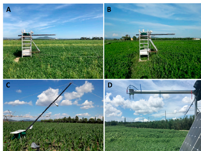
Figure 6. Field measurement set-up over the different targets investigated: (A) forage; (B) alfalfa; (C) corn; (D) chickpea.
