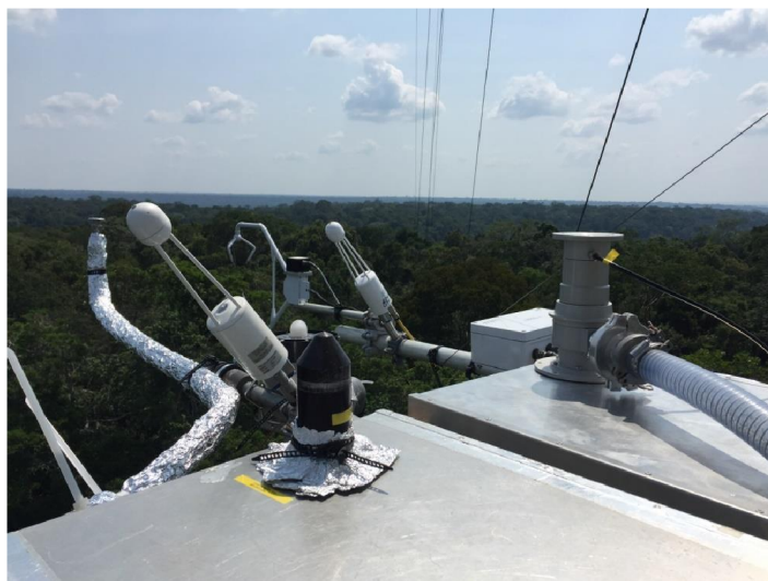
Fig. 1 Set up of instruments and HORUS- inlets at z_R \approx 41\text{ m} at the ATTO tower during ATTO 2015. An inlet pre-injector is mounted on the inlet to the right side of the picture.
