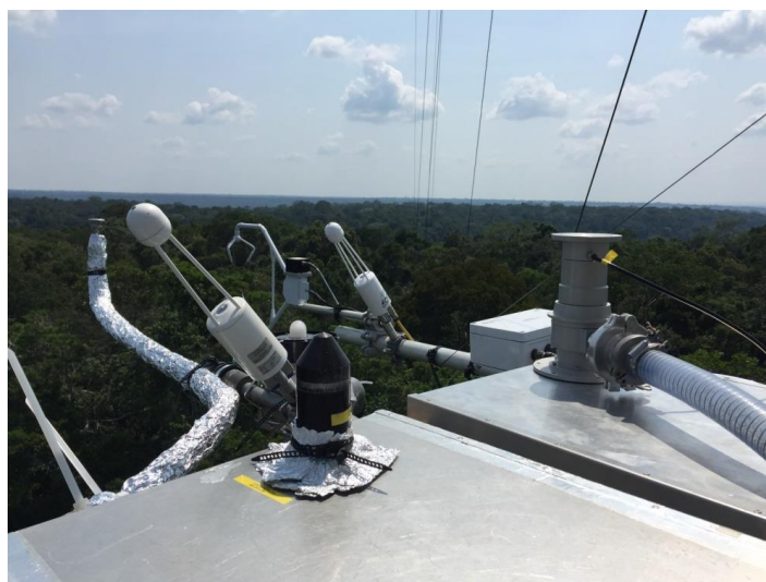
Fig. 1 Set up of instruments and HORUS- inlets at z_R \approx 41 m at the ATTO tower during ATTO 2015. An inlet pre-injector is mounted on the inlet to the right side of the picture.
