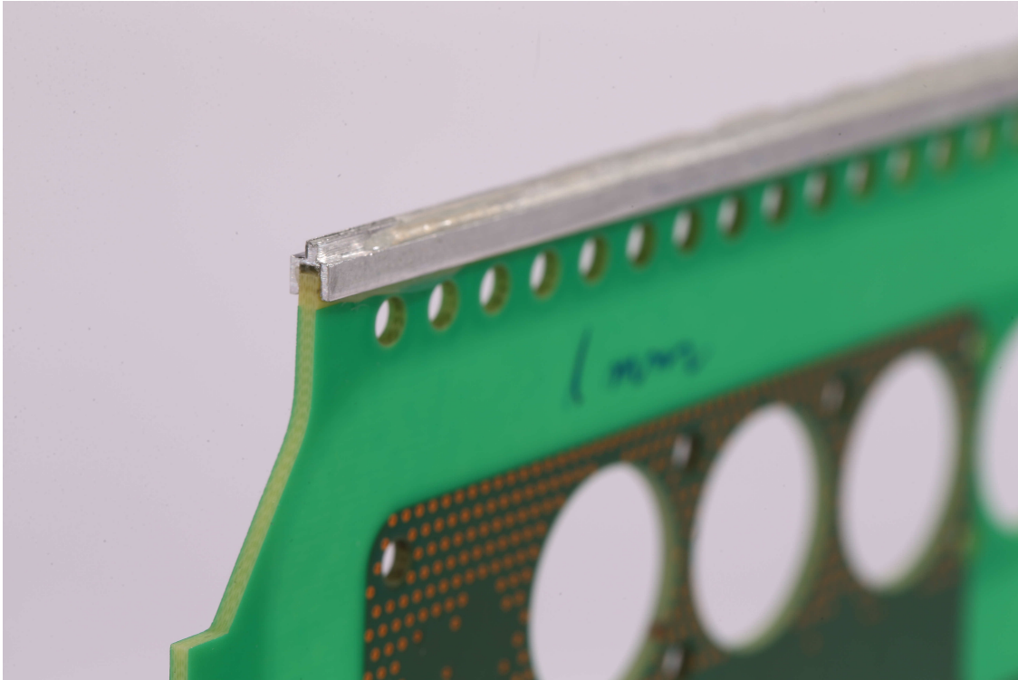
Figure 12: Al Plate Glued to the Top of a GRP Board
