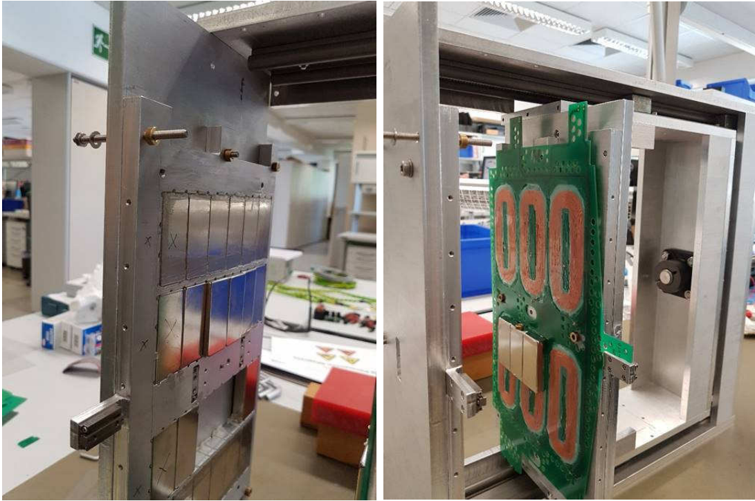
Figure 36: Dislodged Magnets in the 3 Actuator Prototype
