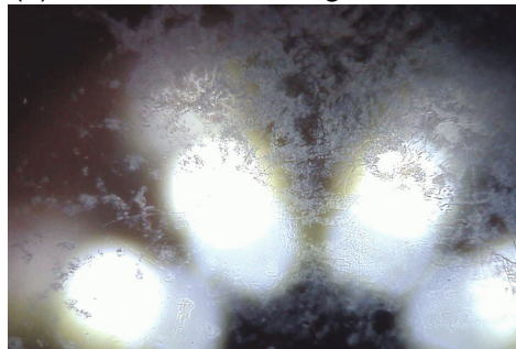
Figure 14. (a) Optical picture of the dry contact between a flat glass surface and the smooth Rubber B's surface. An external force was applied to peel the rubber out of contact with the glass in half of the nominal rubber-glass contact region. (b) A small water droplet was deposited on the rubber surface before the rubber was squeezed in contact with the glass surface. A thin water film separates the surfaces, resulting in the optical fringes seen in the picture. (c) After contact in the dry state, a thin contamination film was deposited on the glass surface. The diameter of pictures is about 1 mm. The white elliptic regions in the figures are due to the eight light diodes used to illuminate the contact.
