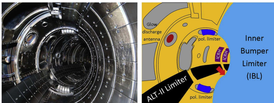
Fig. 1. photograph of the TEXTOR interior and pictorial key to in-vessel components. The red arrow indicates the MoF 6 injection point just behind the Inner Bumper Limiter. View is in direction of the magnetic field under normal configuration. (For interpretation of the references to colour in this figure legend, the reader is referred to the web version of this article.)
