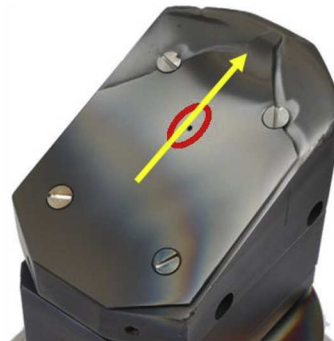
Fig. 14. Local tungsten deposition on the collector plate from the experiment described in [23] comparing Cauchy (red) and Gauss distribution (green). Measurements were conducted along the yellow arrow while the \text{WF}_6 injection point is encircled red. (For interpretation of the references to colour in this figure legend, the reader is referred to the web version of this article.)
