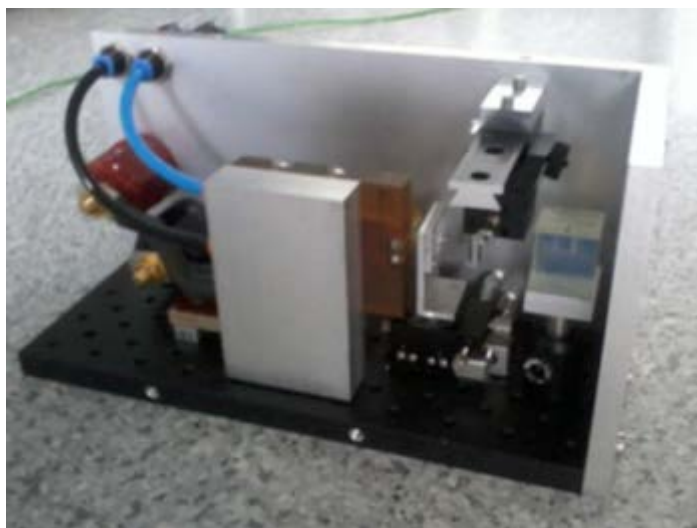
Figure 6. A picture the laser-box of the current volume Bragg grating narrowed laser configuration. This optical setup fit in a custom made enclose box to enclose and mount all the optics and provide connections to power cable and cooling water.
