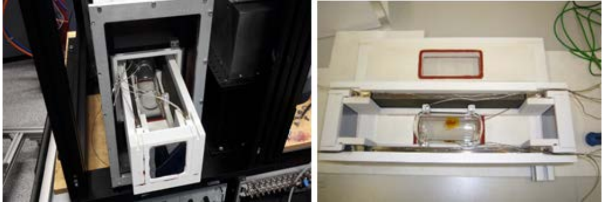
Figure 3. The new oven with He3 cell inside the magnetic cavity
