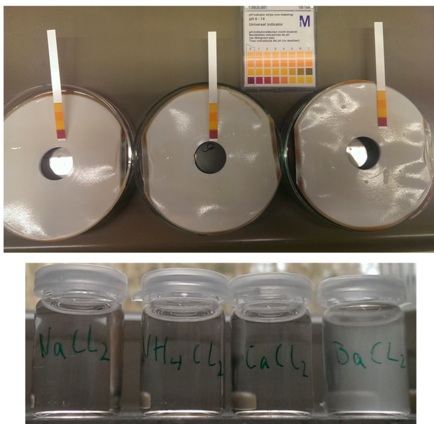
Figure 16. Acidic liquid on SILM envelopes ( top ) proven to contain \text{SO}_4^{2-} (white turbidity ( \text{BaSO}_4 ) in \text{BaCl}_2 ) ( bottom ).
