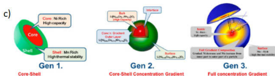
Figure 13. (a) Scheme of full concentration gradient through NMC particle, with Ni-rich core increasing capacity and Ni-poor shell with enhanced structural stability. (b) Scheme of (multilayer-) core-shell NMC particle, with Ni-rich core and Ni-poor shell(s). (c) (Left) Schematic drawings of a core-shell (Gen 1); (center) a Ni-rich core surrounded by a concentration gradient outer layer (Gen 2); and, (right) a FCG lithium transition metal oxide particle (Gen 3) with the nickel concentration decreasing from the center toward the outer layer and the concentration of manganese increasing accordingly. Reproduced from Ref. [122] with permission, Copyright2017, ACS.
