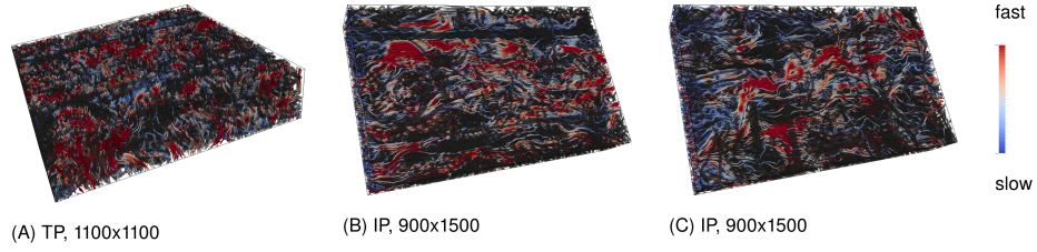
Fig. 5. Transport simulations in stochastic geometry D: (A) through-plane simulation, with the flow direction from the bottom to the top; (B) in-plane simulation amongst fiber bundles, flow direction from left to right; (C) in-plane simulation normal to fiber bundles, flow direction from left to right.
