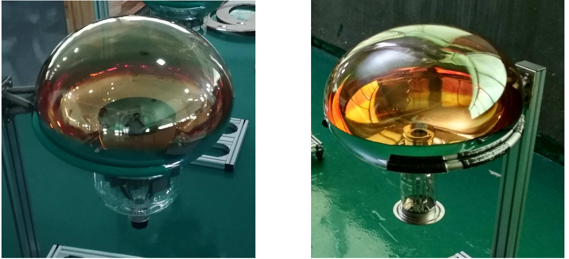
Figure 3.4 – Photographs of the two kinds of 20-inch PMTs that will be mounted in the JUNO CD. The Hamamatsu dynode PMT (left) has a bulkier bottom to accommodate the dynode array. The NNVT MCP-PMT (right) features the reflection photocathode on its bottom half.
