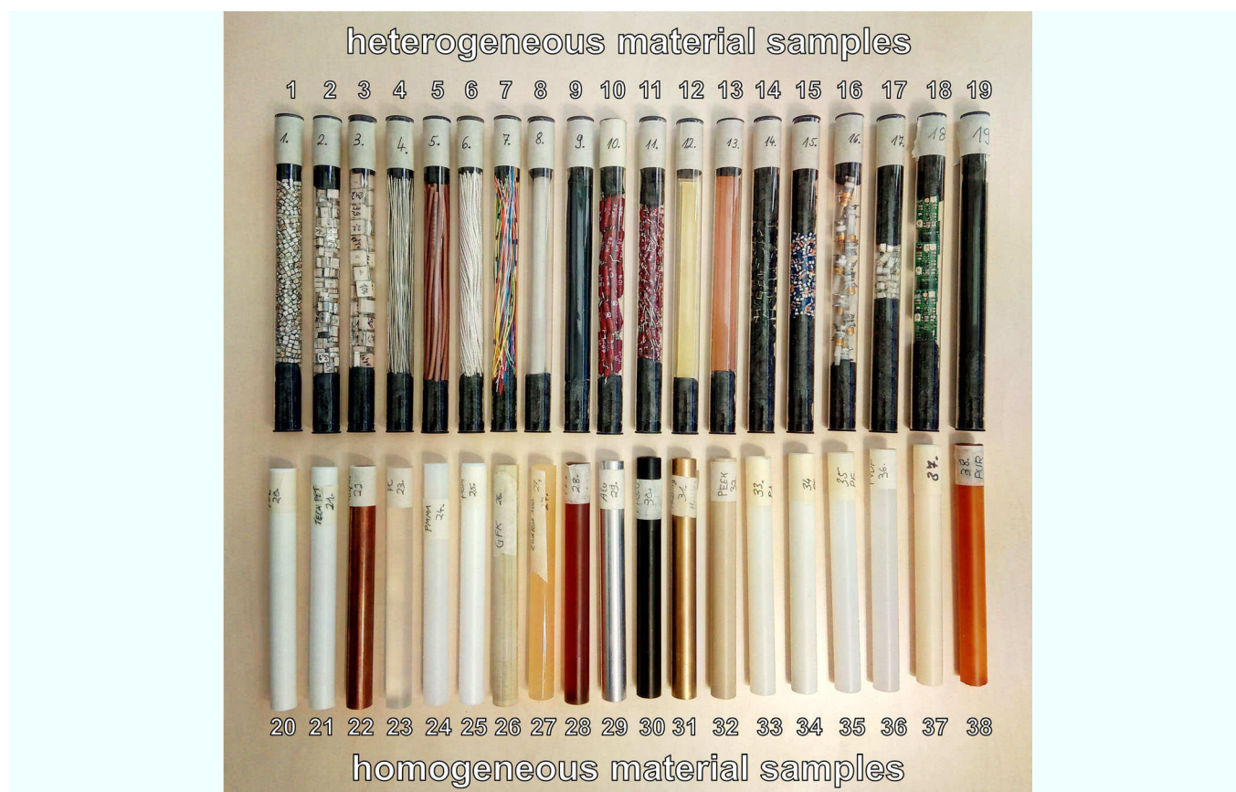
FIG. 1. Overview of all 38 material samples. Samples #1–#19 (upper row) contain several electronic components and cables; samples #20–#38 (lower row) are a collection of various homogeneous plastics and metals. [Color figure can be viewed at wileyonlinelibrary.com ]
