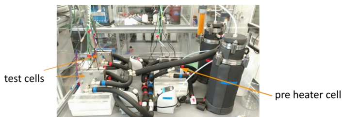
Fig. 58: Photograph of an alkaline test-rig in the newly established laboratory
