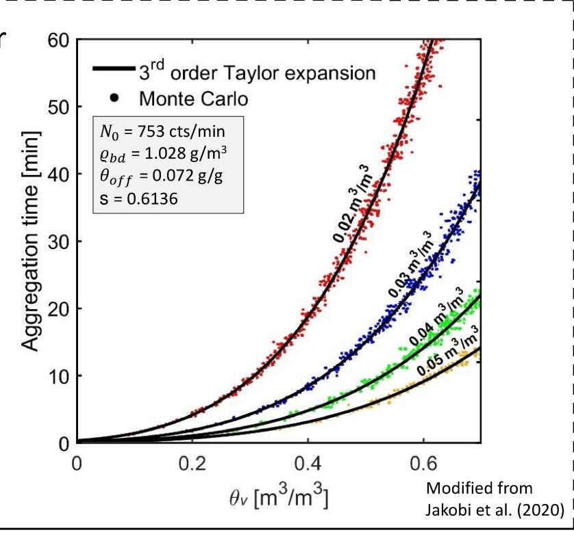
Example of the influence of aggregation on the measurement uncertainty 3 measurements 9 measurements
