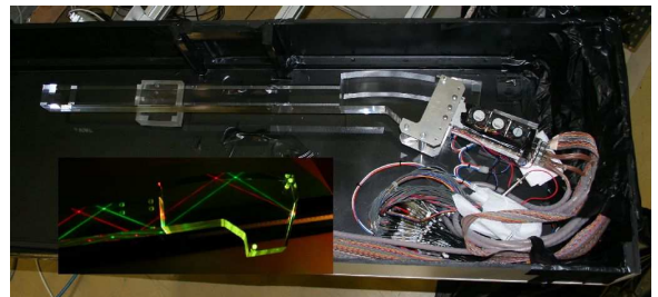
Fig. 15: DIRC prototype radiator with focusing element based on a polynorm shaped surface during beam tests at the COSY-TOF area. The surface treatment was completely done at the Jülich workshop.
