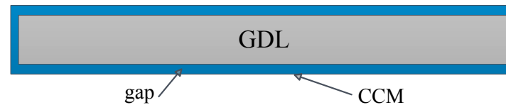
Figure 6.28: The sketch of fuel cells in which the CCM (MEA) is partially covered by the GDL (not to scale).
