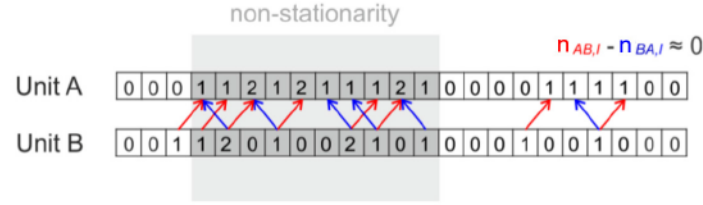
Figure 5.7: CAD pairwise test: Sketch of the statistical pairwise test of the CAD method. The count n_{AB,l} of spikes with a lag l is tested if it is significantly larger than the count at a reference lag. Here the reference lag is chosen equal to -l , which correspond to the count n_{AB,-l} = n_{BA,l} . Under the null hypothesis of independent Poisson processes the observable n_{ABBA,l} := n_{AB,l} - n_{BA,l} has average equal to 0 also in case of firing rate non stationary firing rate. Figure modified with permissions from Russo and Durstewitz (2017).
