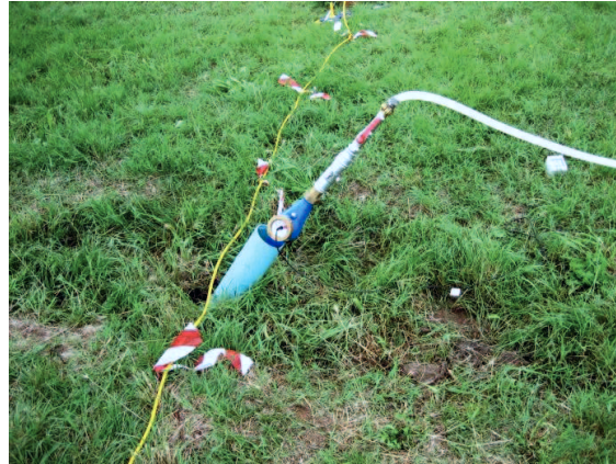
Figure 7.8. Realization of the water injection. Water is infiltrated via an embedded pipe (approx. 2 m depth extension) in order to skip the shallowest soil layer.
