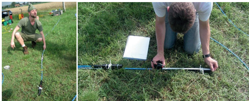
Figure B.2. Preparation of the two-fluxgate array.
