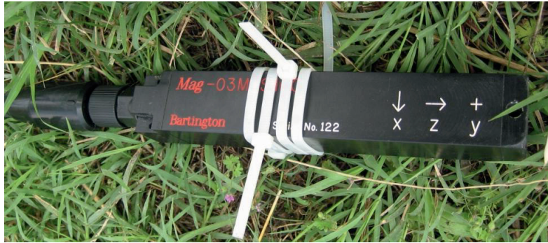
Figure 6.3. Bartington Fluxgate Mag-03. Three-axis borehole sensor with spacers that keep the sensor always in the center of the borehole.
