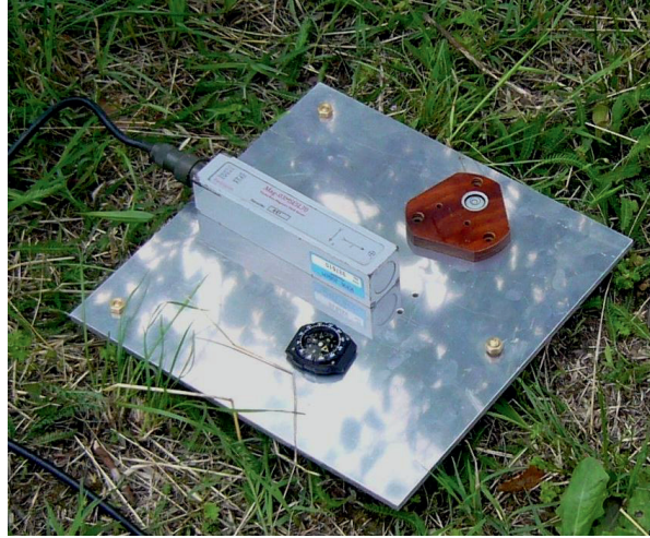
Figure 7.2. Reference sensor (Bartington Mag-03MSSL - low noise version) equipped with level and adjustable feet (not visible here).
