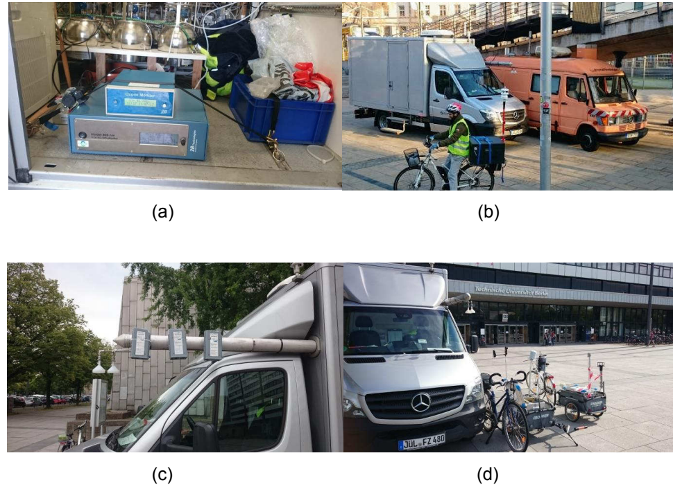
Fig. 5: (a) Ambient air comparison for \text{NO} , \text{NO}_2 and \text{O}_3 with TP8 on the premises of the IFK of the University of Stuttgart (b) Measurement comparison on the Marienplatz in Stuttgart: Mobile bicycle-analytics and stationary-analytics of the IFK with MobiLab-analytics (c) Measurement comparison between MobiLab-analytics and Zephyr probes of the IASS (TP5) (d) Measurement comparison between MobiLab-analytics and mobile analytics of the University of Braunschweig (TP4). The measurement comparisons shown here took place during IOP-II in the summer of 2017.
