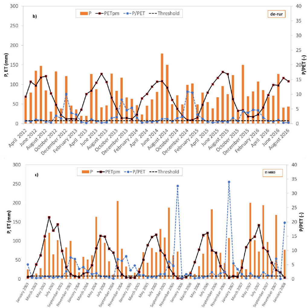
Figure 2. Monthly rainfall, Penman potential evapotranspiration and Budyko Index I = P/PET at Sister site (a), Rollesbroich site (b) and Bondone Mountain (c) for the period under investigation. The threshold of R_n has been set at 2 \text{ MJ/m}^2\text{d}^{-1} .
