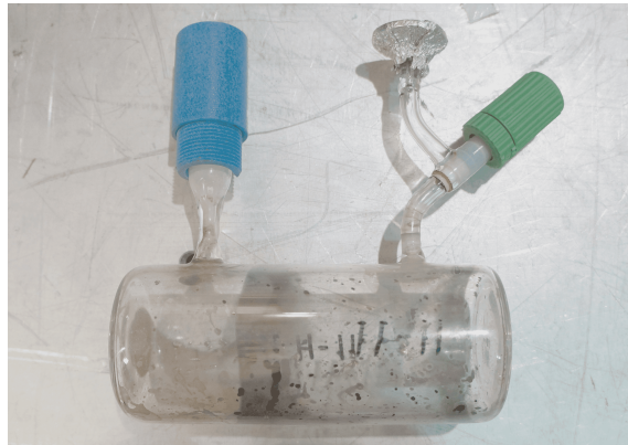
Figure 2. Refillable Cs-coated spin filter cell, made of fused silica.
