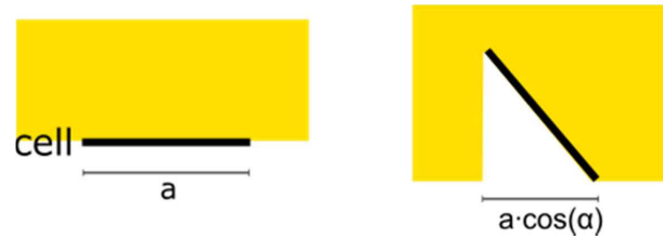
Figure 7.9: Illumination conditions at the current-voltage measurement setup for the evaluation of the influence of varied incident angles. The effective illuminated device area changes according to cosine law (44), taken from reference [132] .
