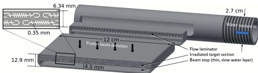
Figure V.41: Basic structure of the internally cooled target
