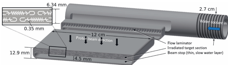
Figure V.41: Basic structure of the internally cooled target
