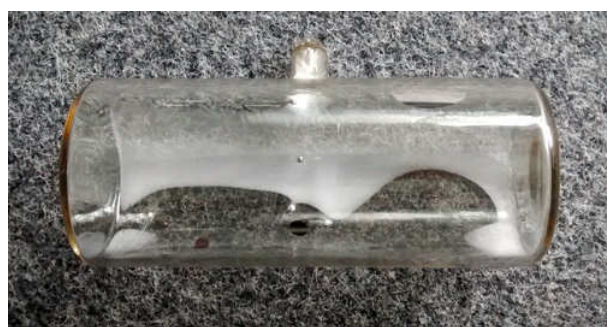
Figure 3. An example of a ^3\text{He} spin filter cell prepared for TOPAS.
