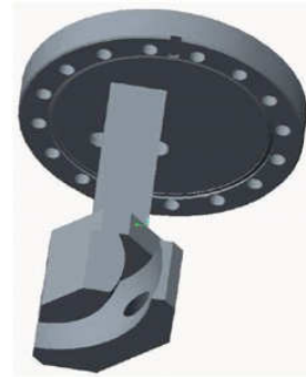
Figure 14. Pulsed electric deflector consisting of two spherically shaped insulated electrodes, one with a hole for the throughgoing beam.
