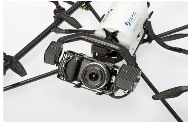
Figure 3. Sony Alpha 6000 camera attached to the Falcon-8 Octocopter.
