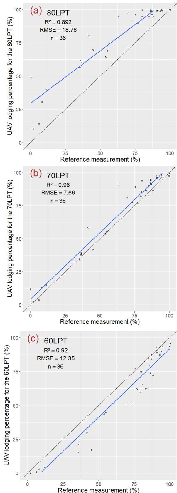
Figure 5. Scatterplots of manually determined lodging percentage (reference measurement) and calculated UAV-based lodging percentage for 80LPT (a), 70LPT (b), 60LPT (c) 75 DAS. Black line represents regression line; blue line represents 1:1 line (n = 36). LPT: lodging percentage threshold; RMSE: root mean square error.
