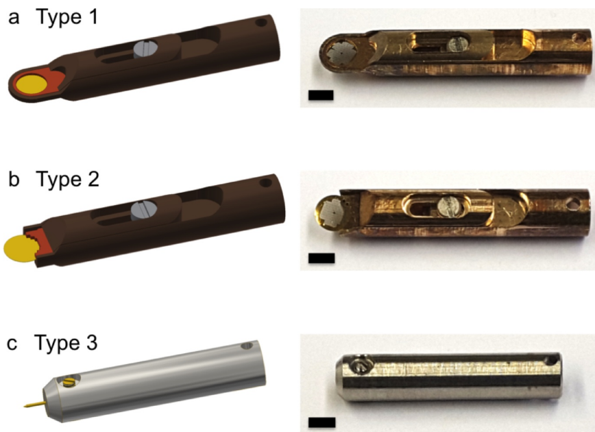
Fig. 2. Schematic diagrams and photographs of three cartridge designs developed for the on-axis tomography specimen holder. The scale bars on the photographs have lengths of 2 mm. (a) Cartridge 1 holds a conventional 3-mm-diameter TEM support grid and has a tilt range of \pm 70^\circ , which is limited by shadowing by the support frame. It can be used for thin or thick samples, including SiN-based membrane chips. (b) Cartridge 2 has a clamping mechanism that provides a full tilt range without shadowing by a support frame. (c) Cartridge 3 is designed to hold needle-shaped samples that have a diameter of 0.25 mm, such as those prepared for characterisation using atom probe tomography.
