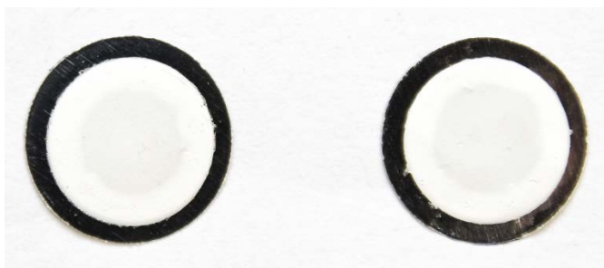
Fig. 1 Photograph of two typical thin ^{86}\text{SrCO}_3 -sedimented layers on Al backing.
