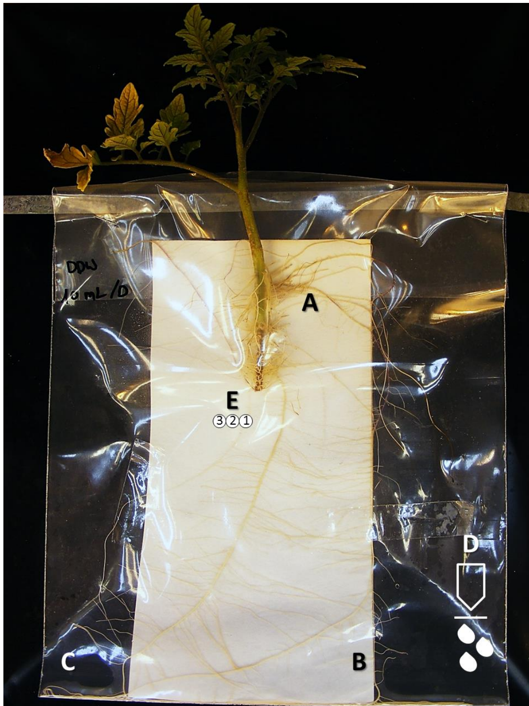
589 Figure 1: Tomato plant growing on a Rhizoslide. The plant (A) is placed on the paper sheet 10X14 cm (B), 590 inside a sealed plastic bag (C), so water can be only transpired. Irrigation is applied through a small cut in 591 the plastic bag (D) with a pipette, without contact with the paper. Na + concentration was sampled from 592 discs (0.7 cm diameter), in growing distance from the root; (1) -0.35-0.35 cm, (2) 0.35-1.05 cm and (3) 593 1.05-1.75 cm (E). The bags are placed in a box to keep the roots in the dark.
