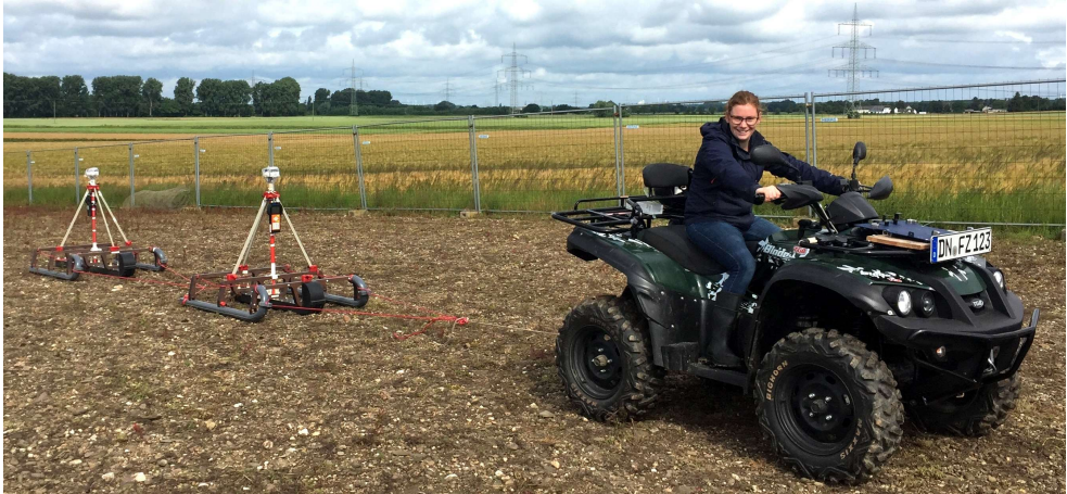
Figure 5: Example of the EMI measurement setup. The ATV is used to pull the CMD MiniExplorer (first plastic sled) and the CMD MiniExplorer Special Edition (second plastic sled). A GPS/DGPS unit that is connected to the EMI device is positioned on top of each sled.
