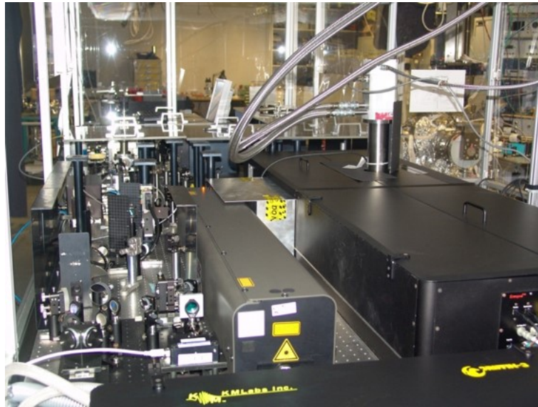
Figure 9: Multi-pass laser amplifier (KMLabs) providing 2 mJ pulse energy at 3 kHz forms the core of the Ju SPARC_DENEB laser system commissioned for spin dynamics experiments in thin magnetic films and multilayers.
