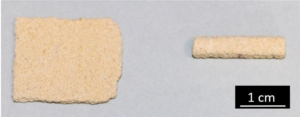
Fig. 1. The visualization of samples of Maastricht limestone used for SANS (on the right) and \mu -CT testing (on the left).
