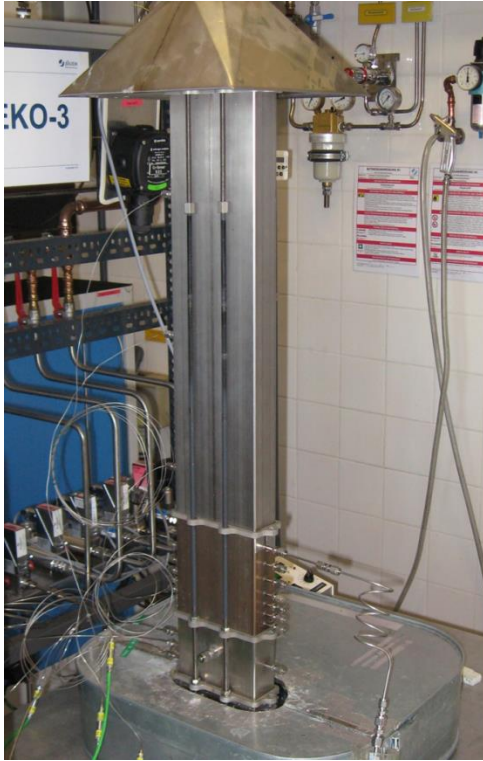
Figure 1. REKO-3 experimental set-up: Rectangular flow channel (left), catalyst sheets equipped with thermocouples (right).
